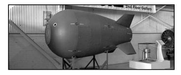
The bomb was blimp-like in its design – 3.25 meters long and 1.5 meters wide. It weighed five tons. According to the United States Air Force (USAF,) the bomb did not contain the plutonium core necessary for a nuclear detonation.
